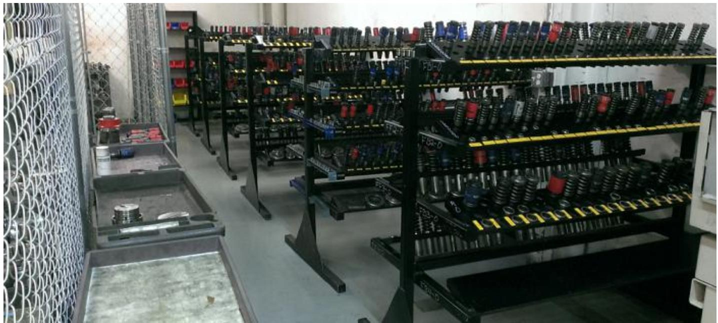
One of the kaizen projects involved reorganizing and creating a management system for the turret punch tool center. The improvement enhanced the efficiency and workflow of the turret punch cells and facilitated maintenance and inventory improvements.
