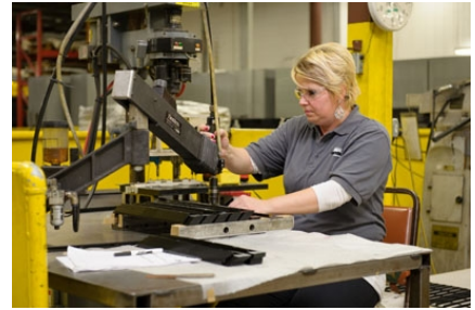
Senada Ibrahimovic using a tapping arm to thread holes in a part
